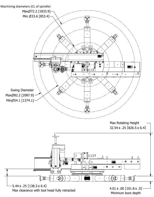
ID Chuck Assembly, ID-Mount Configuration, Milling
