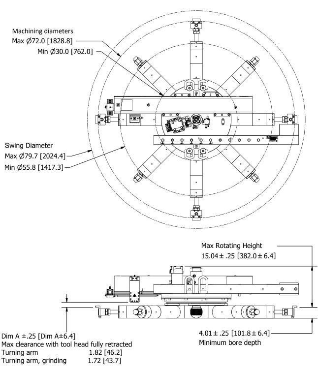
ID Chuck Assembly, ID-Mount Configuration, Single-Point Machining
