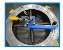
Select the appropriate leg length and foot. Install setup fingers.
